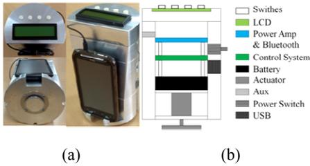
Fig. 4 Photography of docking speaker(a) schematic design(b)
