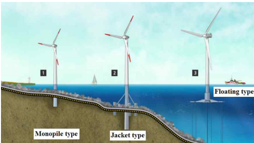
Fig. 1 Types of offshore wind farm construction
