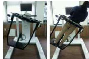
Fig. 1 Driving type of 3-D dynamic system (left ; passive type, right ; active type)
