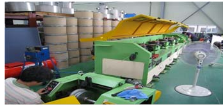
Fig. 1 Pilot line for the production of metal cored welding wire
