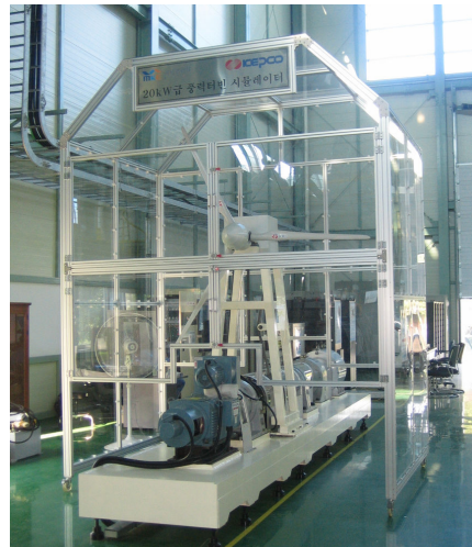
Fig. 1 20kW Wind Turbine Simulator
