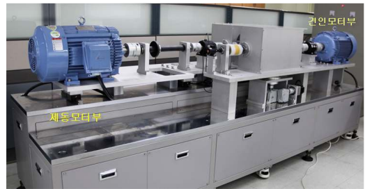
Fig. 1 Scaled adhesion tester for analyzing the adhesion characteristic
