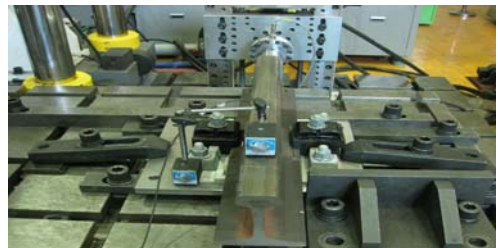
Fig.1 Rail longitudinal Force Testing
