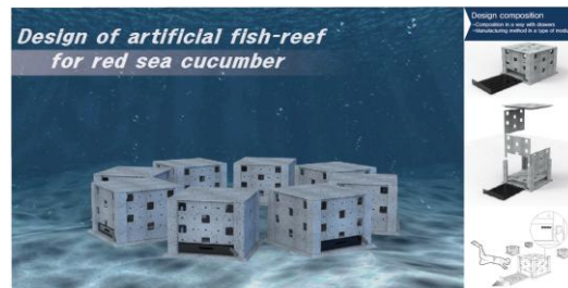
Figure 2. Design of artificial fish-reef for red sea cucumber
