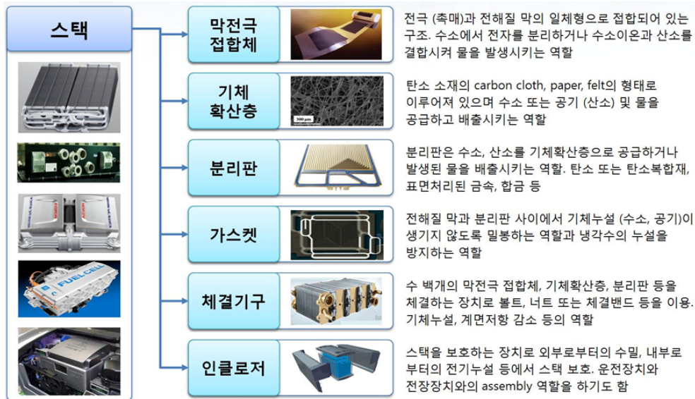
Fig. 1. Fuel cell stack components
