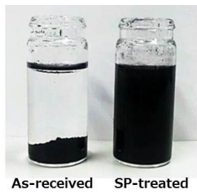
Fig. 1. Image of (a) as-received MWCNTs (b) SP-treated MWCNT
