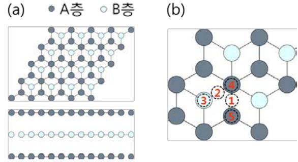
Fig. 2. (a) Clean graphene  $4\times 4$  super cell의 topview와 sideview. (b) Ne 원자를 adsorption, intercalation시킬 위치.
