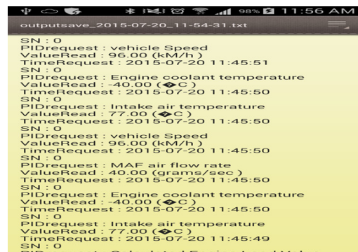
Fig. 4 File of Vehicle performance data saved on the SQLite database management on the car owner mobile device
