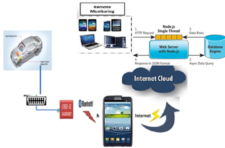
Fig. 1 System design of mobile vehicle diagnostics system with Node.js at web side
