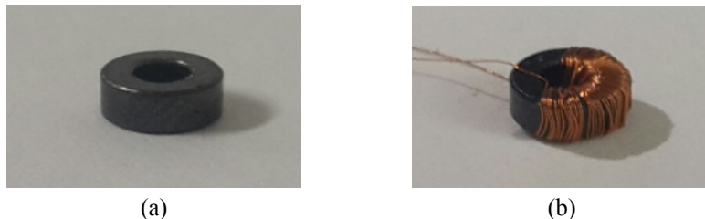
Fig 1. Photographs of ferritecore(a) and toroid sample(b)
