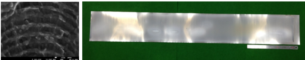
Fig. 1. Cross sectional view of Al-Ni layers and nano foil sheet
