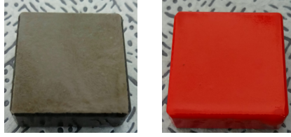
Fig. 2 sample shape of teflon(PTFE) coating and marine paint coating.
