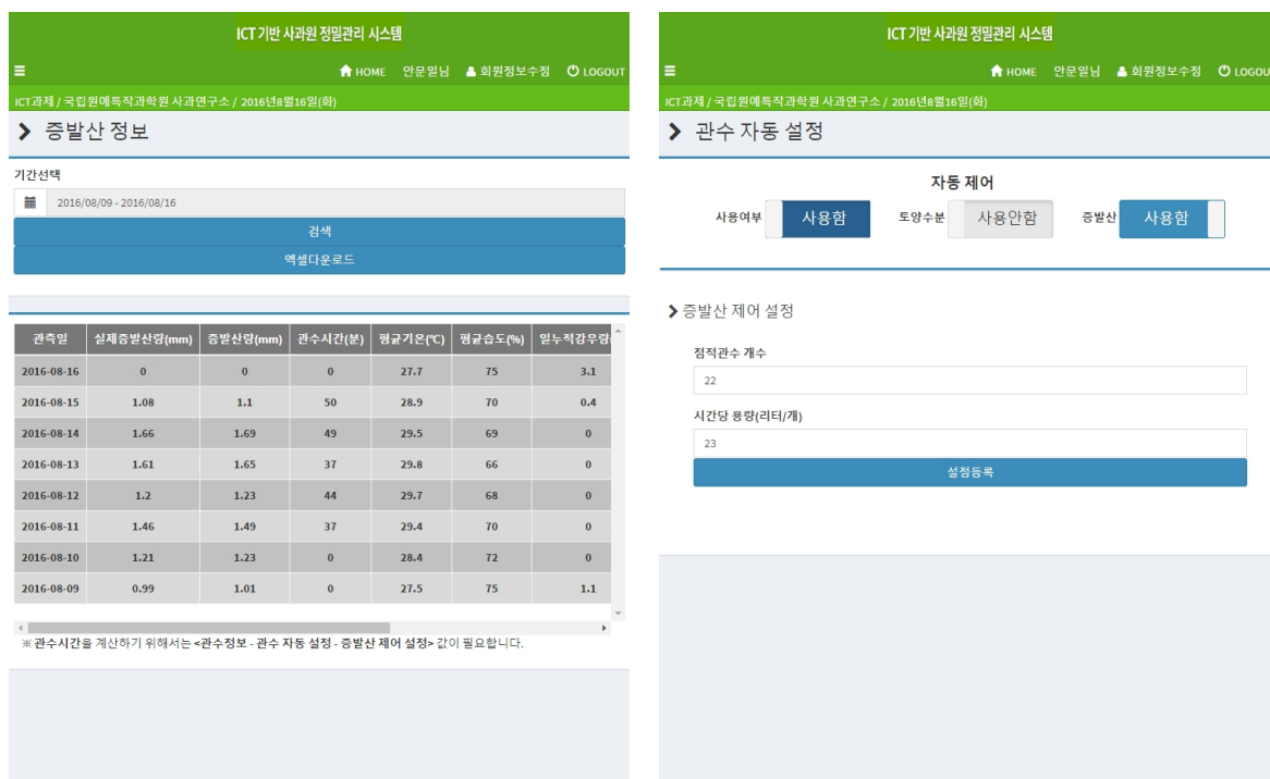
Fig. 6. Screenshots of evapotranspiration predictions using ICT-based environmental measurements, and the irrigation control system that utilizes these predictions.
