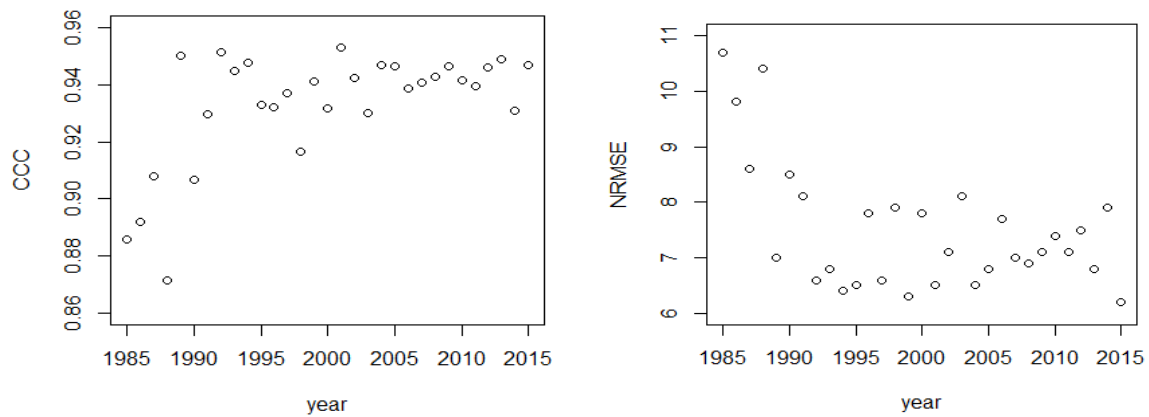
Fig. 2. Concordance correlation coefficient (CCC) and normalized root mean square error (NRMSE, %) between observed and estimated solar radiation using the Angstrom-Prescott model by year.
