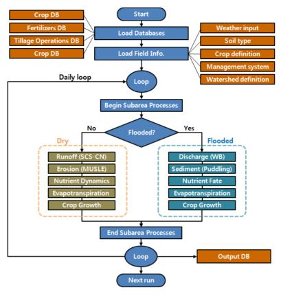
Fig. 1. Paddy algorithm of APEX model.
