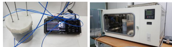
Fig. 2. Measuring the heat-generating temperature of the solidification depending on the curing temperature– Room temperature (L), 50 °C atmosphere (R).
