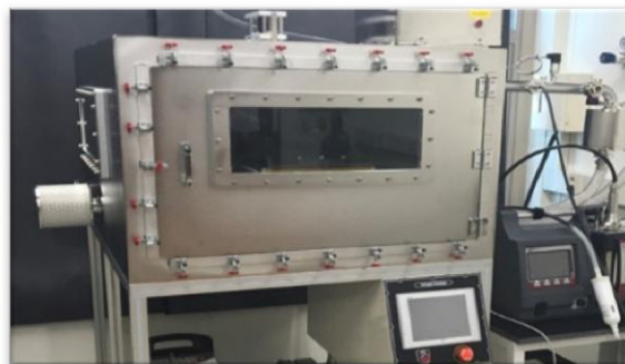
Fig. 1. The aerosol system for the measurement of physical and chemical characteristics of aerosol.
