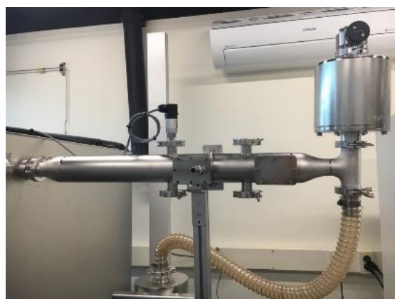
Fig. 2. Sampling pipe and measurement lines.
