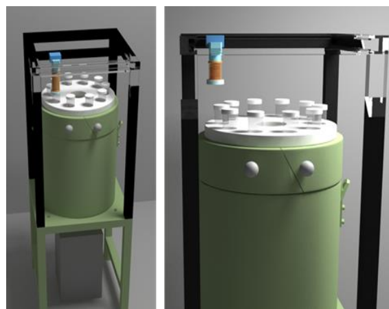
Fig. 1. Automated sample feeder for gamma spectroscopy system.
