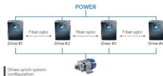
Fig. 1. Drives synch system configuration.
