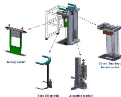
Fig. 2. A modular design of the basket lifting mechanism.
