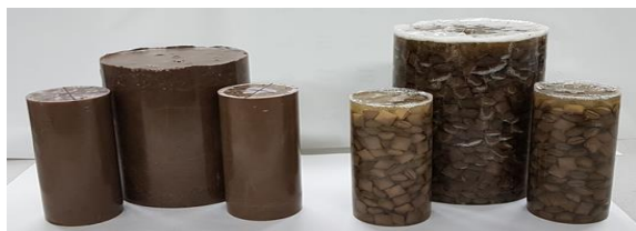
Fig. 3. Powder Solidification agent(L) and Pellet Solidification agent(R).
