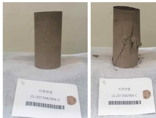
Fig. 1. Compressive strength test of specimen (before/after).
