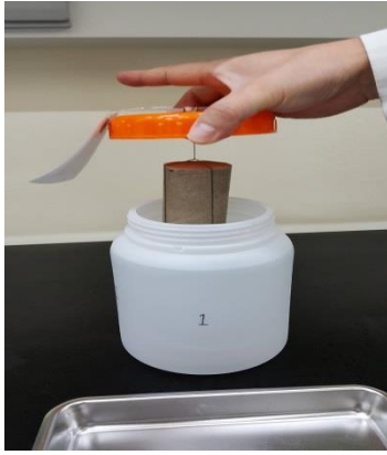
Fig. 2. Immersion and leaching test.
