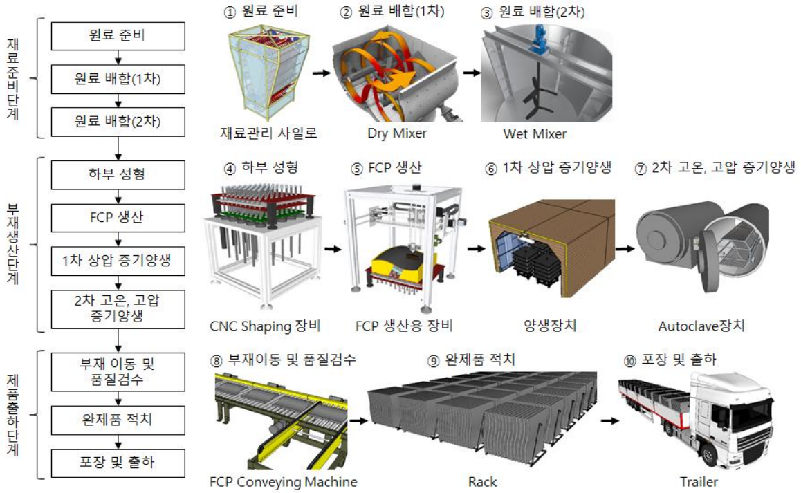
그림 2. Production system of freeform concrete panels
