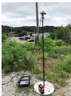
(a) Measured by attaching a skywave reduction cap to the implemented loop antenna
