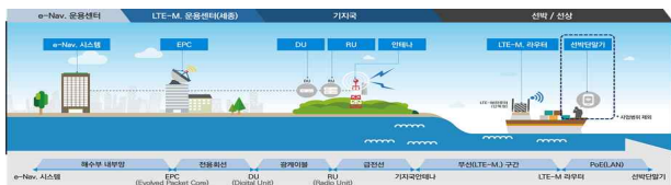
Fig. 1 LTE-Maritime system configuration
