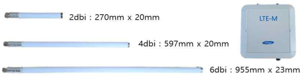
Fig. 3 Prototype router and 2/4/6dbi antenna
