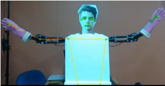
Fig. 2. Extracting the robot's joint coordinate values using MPP (simple pose)
