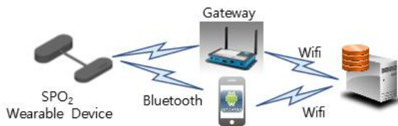
Fig. 3. Proposed SPO 2 Wearable device
