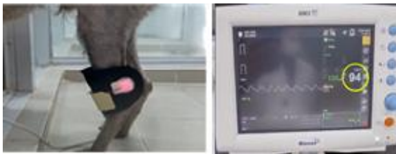
(a) Attachment location for the SPO 2 wearable device (b) Measured results in connection with existing devices
