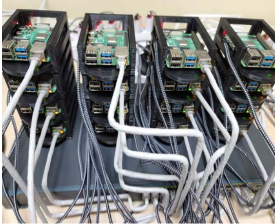
Fig. 1 Raspberry Pi 4 Cluster
