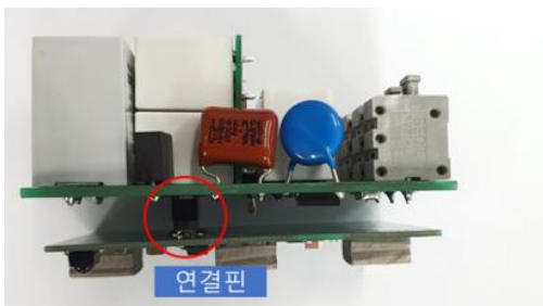
Fig. 2. Power Board and Controller Board
