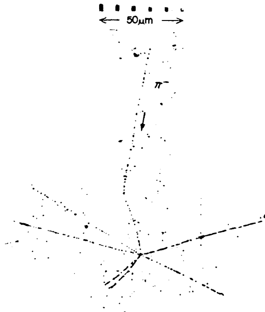
Fig. 2. Star formed in photographic emulsion by \pi meson capture by an oxygen nucleus.
