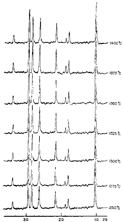
Fig. 3. X-ray diffraction patterns of KTN specimens.
