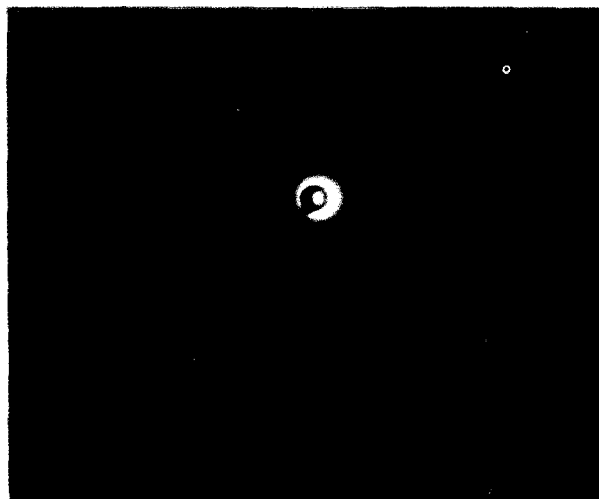
Figure 3. Typical small-angle diffraction pattern of surfactant, Sunsoft O-30B
