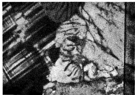
Sec. 30-1 : Microcline, quartz and feldspar were scattered by stronger stress, crossed nicol, X30
