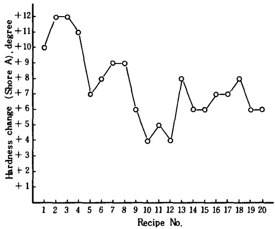
Fig. 3 Comparison of hardness change after Aging, 100 °C × 70 hrs.
