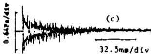
Figure 4. Waveforms by impact. (a) force, (b) acceleration, (c) sound pressure (ball diameter d=10\text{mm} , dropping height h=250\text{mm} , thickness h'=20\text{mm} )
