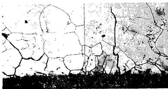
(a) 650°C, ×300 Δε p =0.40% f=25.6 cpm (b) 650°C, ×300 Δε p =3.32% f=5.1 cpm
