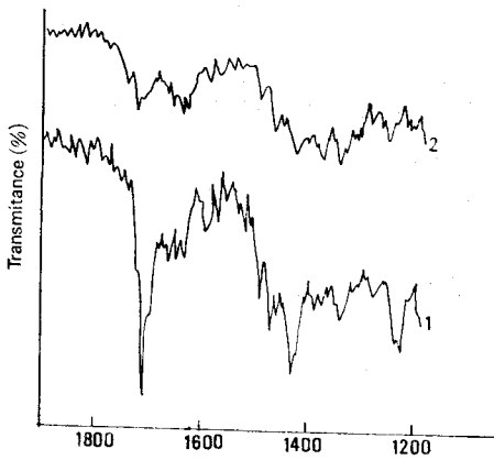
Figure 4 —IR absorption spectrum of flurbiprofen/ \beta -CyD according to KBr disk method. Key : 1, flurbiprofen- \beta -CyD complex; 2, flurbiprofen- \beta -CyD physical mixture
