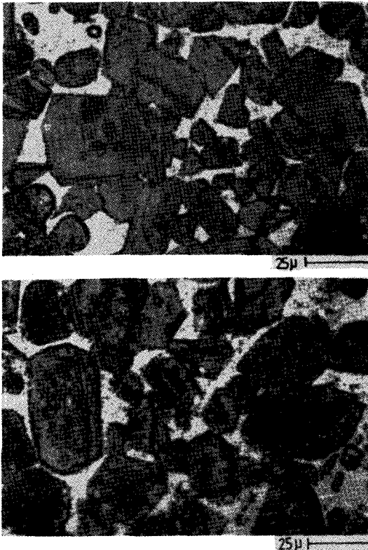
〈그림-3〉 Optical micrographs: synthesized clinker (upper). commercial clinker (lower).
