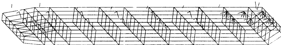
Fig. 3 Structural model of Heerema Barge and distribution of tie-downs
