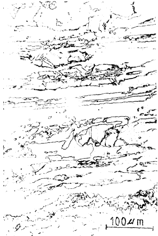
Fig. 1 Microstructure of duplex stainless steel (SUS329J)
