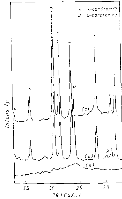
Fig. 8 X-ray diffraction patterns of cordierite powder prepared at 800°C : (a) as-prepared, (b) calcined at 1000°C for 2 hrs. and (c) calcined at 1300°C for 2 hrs.
