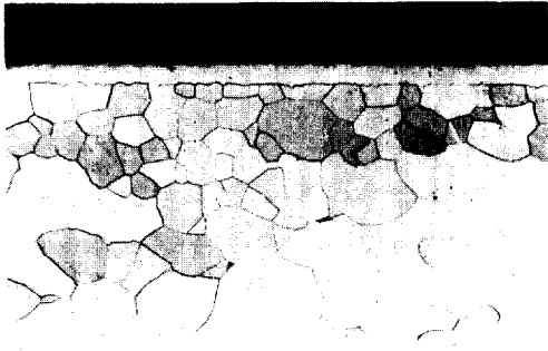
Fig.1 Optical micrograph of pure iron after gaseous nitrocarburizing treatment for 3 hours at 570°C, followed by oil quenching.
