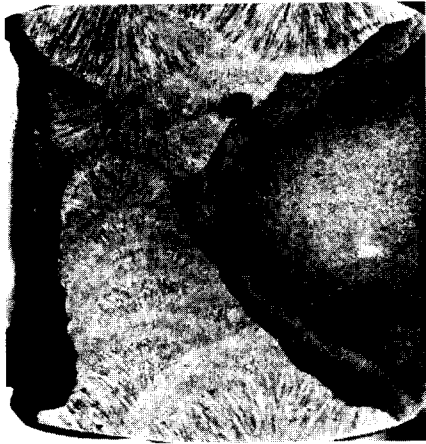
Photo. 1 Macroscopic cross sectional view of the welded joint
