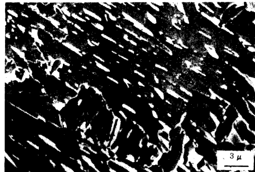
Photo. 4 Scanning electron micrograph in the simulated ICRCG HAZ prepared by the 2-stage electrolytic etching technique 12) to observe M-A constituent
