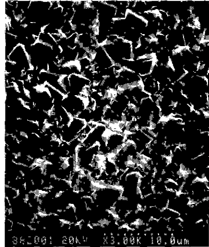
Fig.4. SEM micrographs for the microwave plasma CVD diamond deposited on silicon wafer at the following conditions : microwave power ; 500 W, methane ; 0.7%, pressure ; 40 torr, total flow rate ; 60 sccm.
