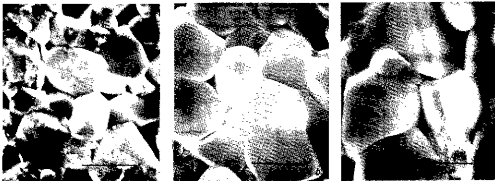
Fig.12. SEM photographs of spinel specimens sintered at each temperature for 1hr. (a) 1,600 (b) 1,650 and (c) 1,700℃.
