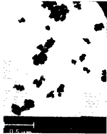
Fig.11. TEM of powders leached (mullite).
