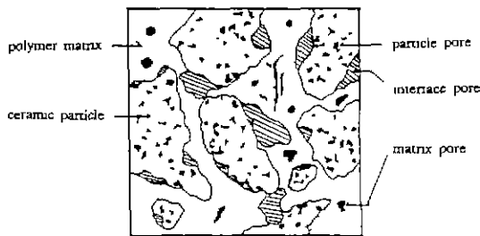
Fig.2. Microstructure of composite with three kinds of pore.
